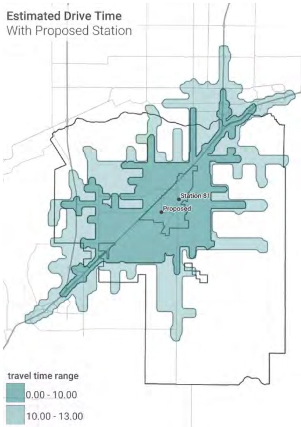
To put the fire protection system into perspective, the following map illustrates the travel time using the proposed new station and including the automatic aid partners. The travel time used was the rural demographic of a 10-minute benchmark and 13-minute baseline travel time.
